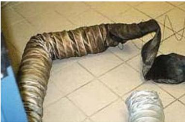
Fires originated most frequently from two places: dryer venting and the lint trap, due to improper vent cleaning and the use of improper dryer venting.
